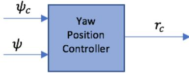
Figure 6. Block diagram of yaw position controller
