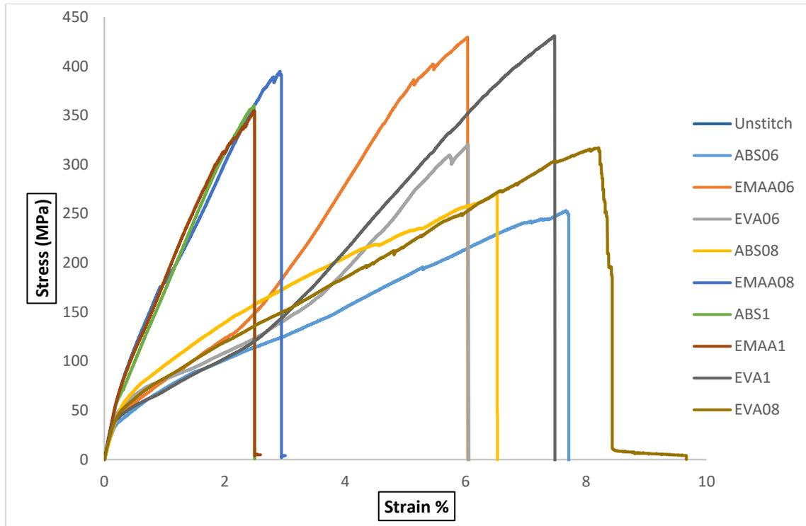
**Figure 2.** Stress-strain curves of composite materials produced with different filament diameters
