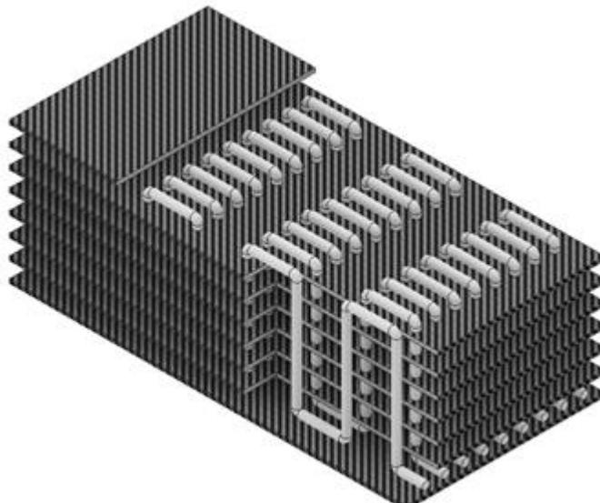
**Figure 1.** The demonstration of the stitches in the carbon fibre–epoxy composite
