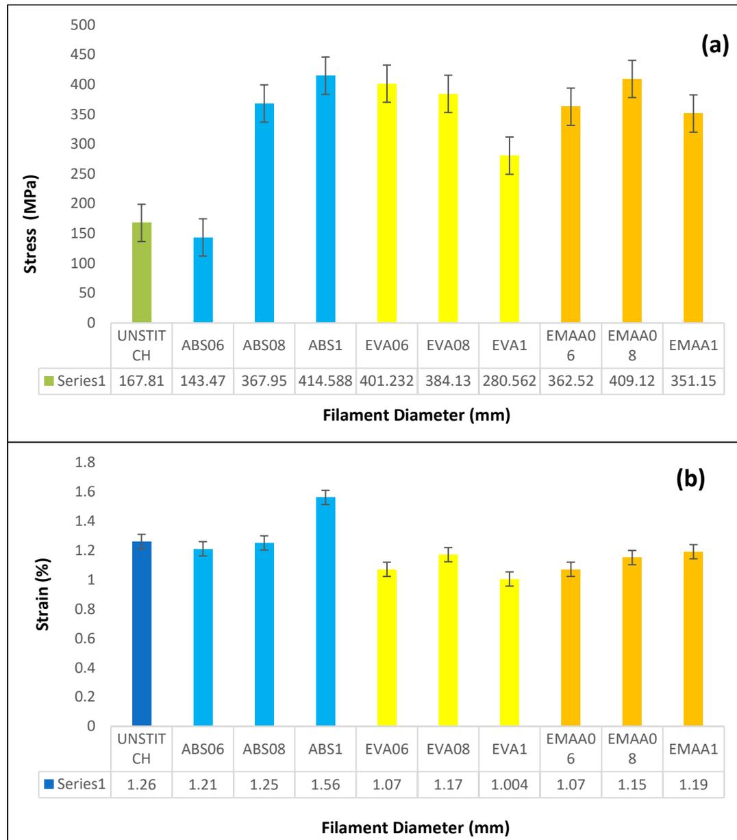
**Figure 3.** The variation of the stress(a) strain(b) graphs obtained as a result of the three-point bending test of the composite materials prepared with ABS, EMAA, and EVA filaments according to the filament diameter
