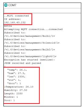
Figure 8. Sensors reading data on the serial monitor
