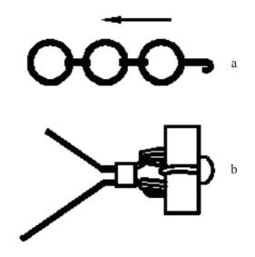
Figure 2- Top view diagrams of covering components (a, chain type; b, spring type)
