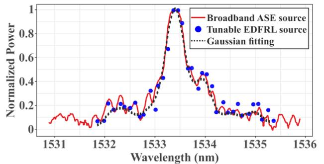
Figure 4 Measured reflection spectrum of the FBG sensor at room temperature (25°C) with a broadband ASE source and a narrow linewidth tunable EDFRL source as interrogator and Gaussian fitting curve of the points.
