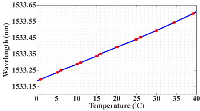
Figure 5 Linear response of the FBG sensor to temperature variation from 0°C to 40°C with broadband ASE source interrogator.
