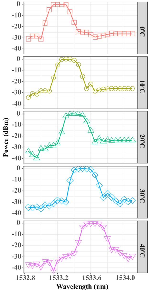
Figure 6 Reflection spectra of the FBG temperature sensor for different temperature values. Here, the interrogator is a narrow linewidth tunable EDFRL source.
