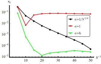
Figure 4.  $\epsilon_k$  values of the node number dependent shape parameter,  $\alpha = 1$  and  $\alpha = h$  approaches for the 3-group fission source problem
